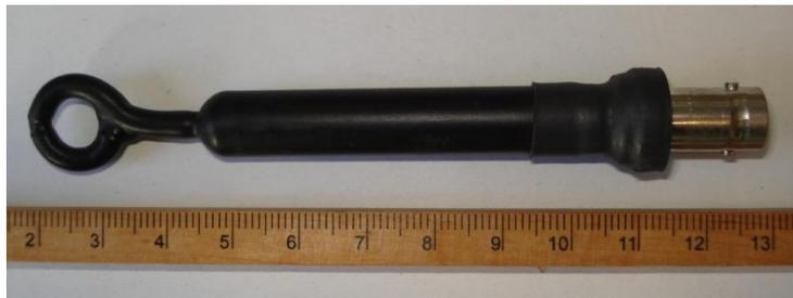
**Figura 4.16: Sonda EM6995 de Electro-Metrics**
